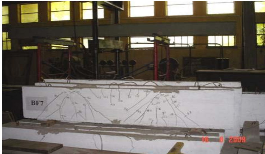
Beam Specimen after Testing
