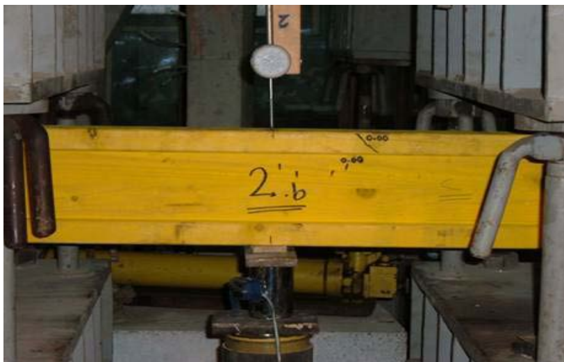
Wooden Beam Loading Test
