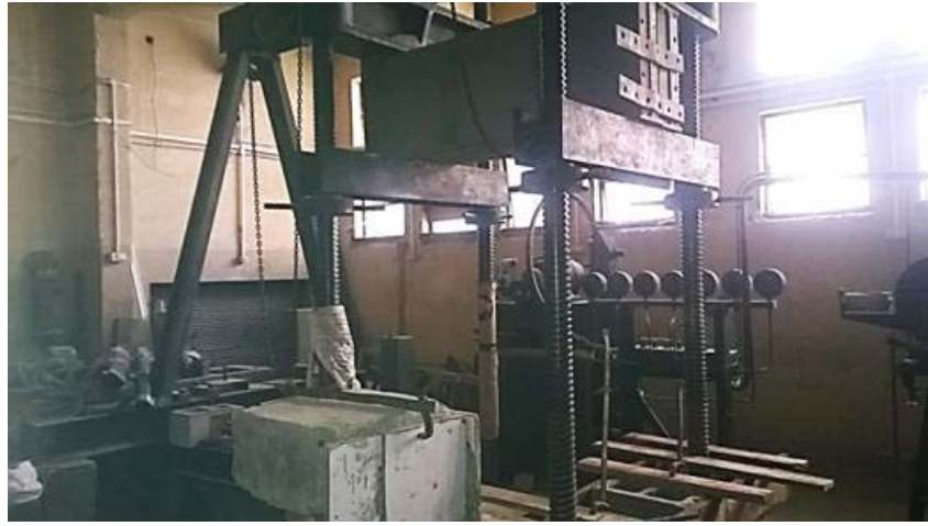
175 ton Hydraulic Testing Machine
