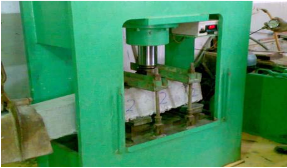
Railway Beam Loading Test
