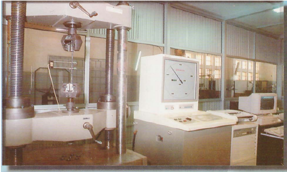
Computerized 50 Ton Shimadzu Universal Testing Machine
