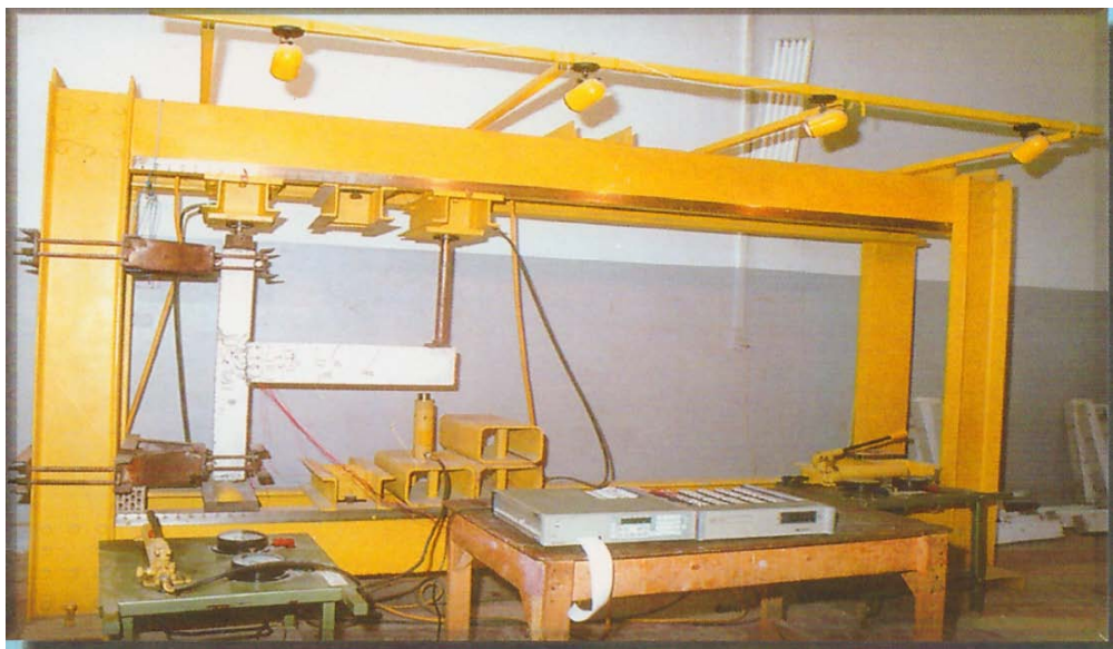
40 Ton Loading Frame for Testing Non-Standard Models
