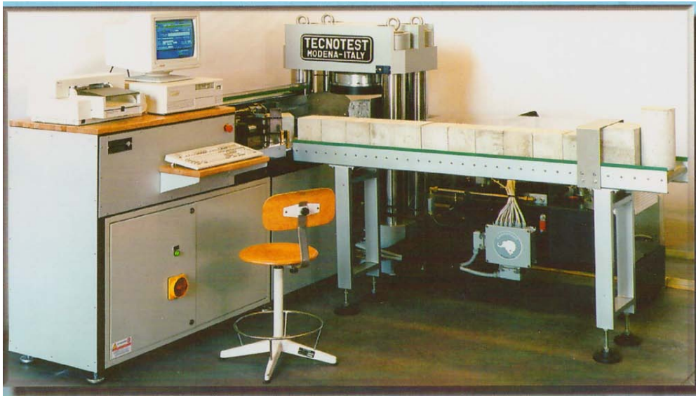
Computerized 400 Ton Technotest Compression Testing Machine
